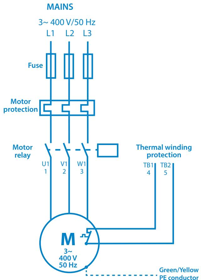
Connection of the thermal winding cover:
